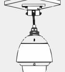
3. Fix with tightening screw, thread the cable and install the speed dome
