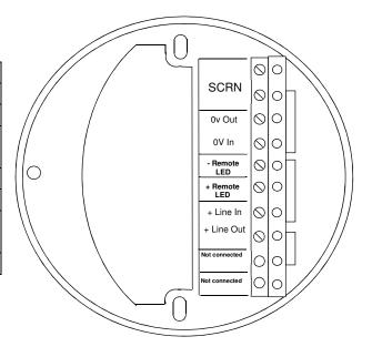
Remember that the device at the end of the line must have its EOL signal activated using the relevant DIL switch. Do not use a resistor or capacitor (or another manufacturer's End of Line device) as the end of line, as this may prevent correct operation of the zone.
