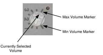
NOTE: that the minimum volume which can be set is no sound. Care should therefore be taken when setting up a sounder for very low volume. In any case, it is important to ensure that sound volumes meet all regulatory requirements for your installation.
